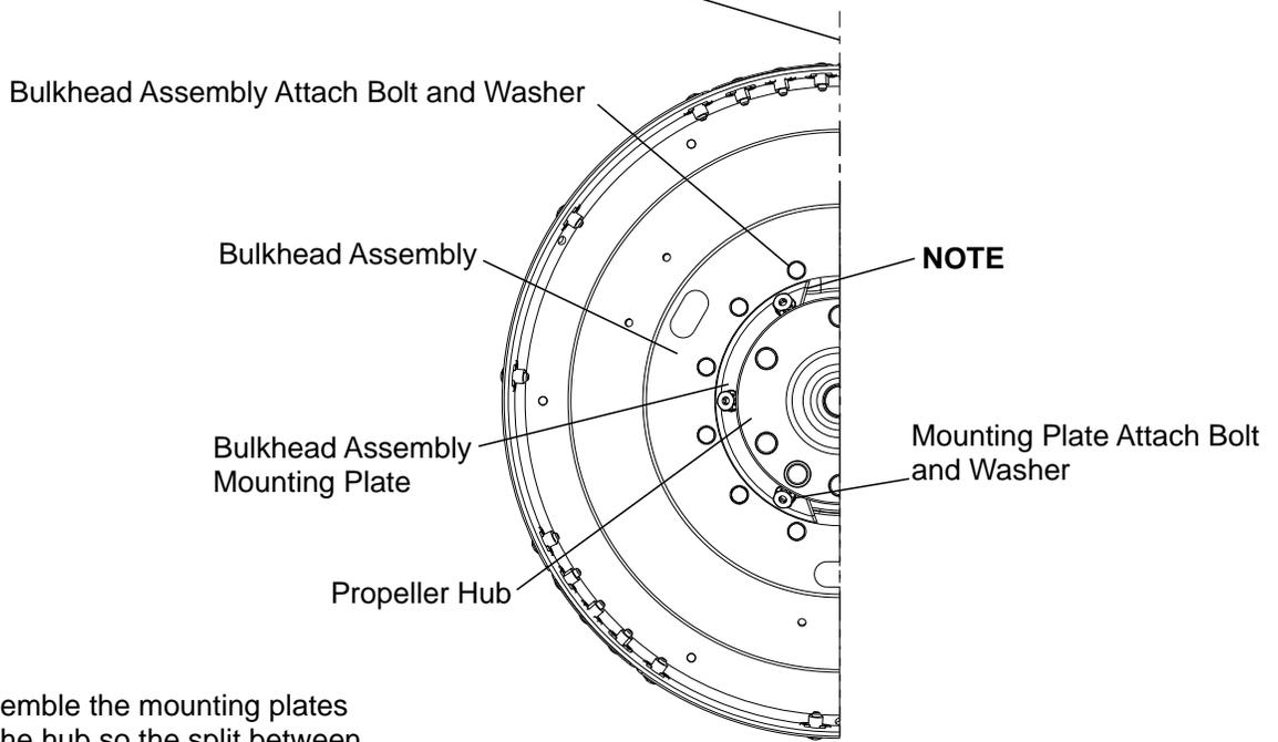
**NOTE:** Assemble the mounting plates on the hub so the split between the mounting plates is in line with the centerline of the number 1 propeller blade.
